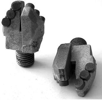
Cutters for rotary drilling holes equipped with working elements of diamond-tungsten carbide polycrystalline composite
